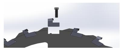
Keystone's patented Dowel-and-Pin System securely locks the tool to the blade; increasing the life of the blade and the tools
