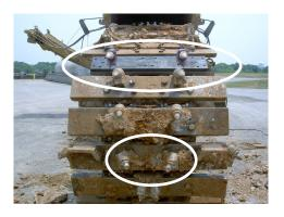
Keystone's bolt-on trenching plate allows you to position toolholders to maximize cutting efficiency, dramatically improving tool and chain life and reducing vibration on the machine
