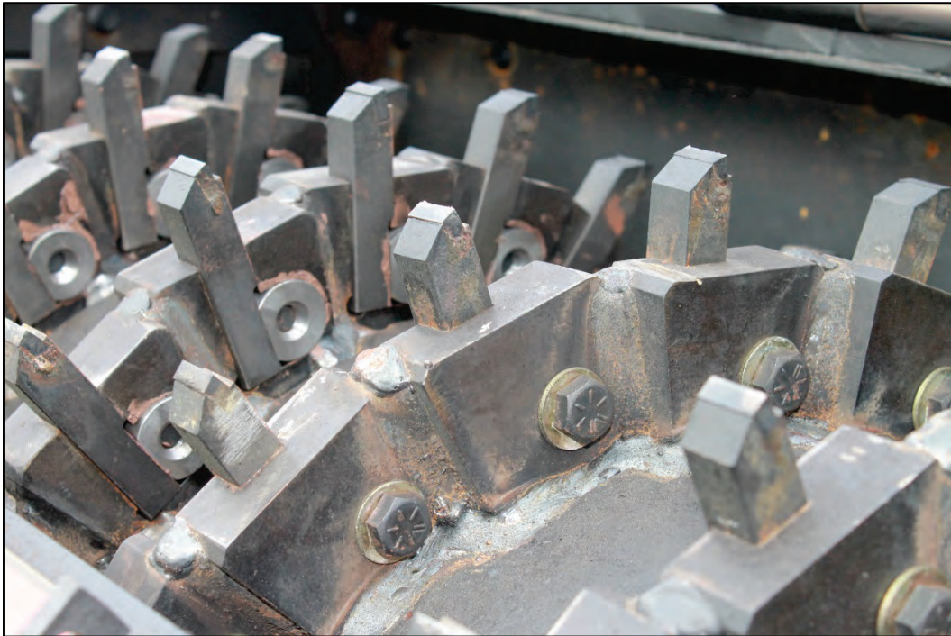
Figure 37. Close up view of the Flatliner bits and housing.
