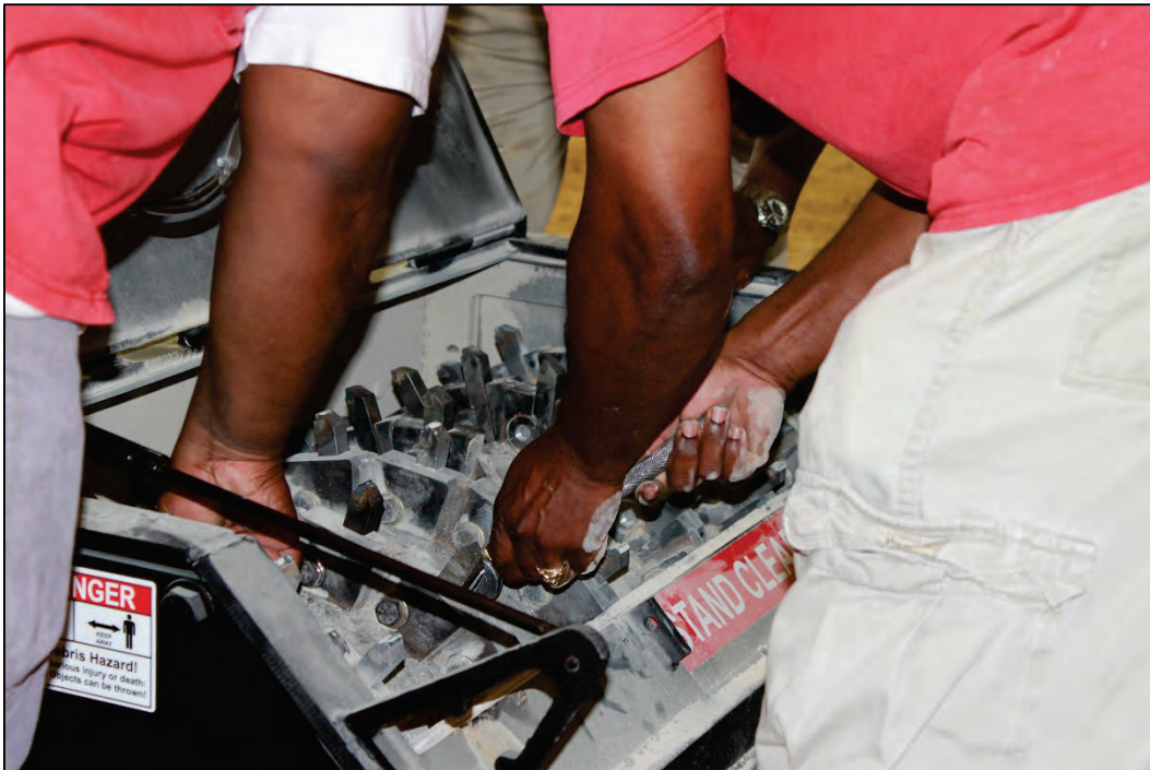
Figure 36. Replacing bits on Flatliner's drum.
