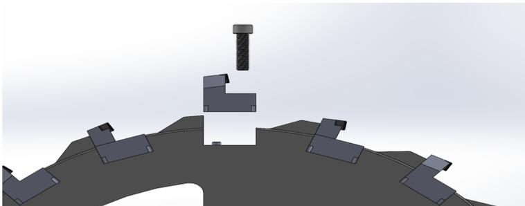
Keystone's patented Dowel-and-Pin System securely locks the tool to the blade; increasing the life of the blade and the tools
