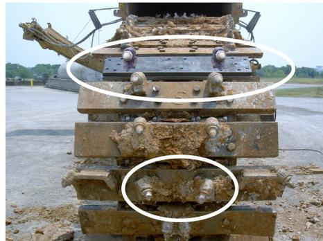
Keystone's bolt-on trenching plate allows you to position toolholders to maximize cutting efficiency, dramatically improving tool and chain life and reducing vibration on the machine
