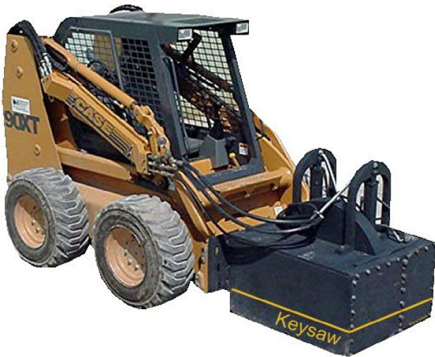
Skid Steer Attachment Designed for Longitudinal Joint Repair
