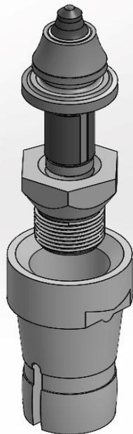
EZ303 Tool Holder with Standard Carbide Tool and Replaceable Insert
